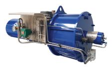
**ALGA-ALGAS pneumatic scotch yoke actuators** are suitable for quarter-turn valves up to the largest sizes, thanks to an efficient design and to high break-out torque. The QA version with damper performs fail stroking in less than 1 second.
