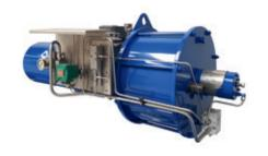
ALGA-ALGAS pneumatic scotch yoke actuators are suitable for quarterturn valves up to the largest sizes, thanks to an efficient design and to high break-out torque. The QA version with damper performs fail stroking in less than 1 second.
