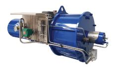
**ALGA-ALGAS pneumatic scotch yoke actuators** are suitable for quarter-turn valves up to the largest sizes, thanks to an efficient design and high break-out torque. The QA version with damper performs fail stroking in less than 1 second.
